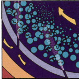
Micronizer®: Jet mills dry particles to sub-micron size; some models USDA-accepted.
