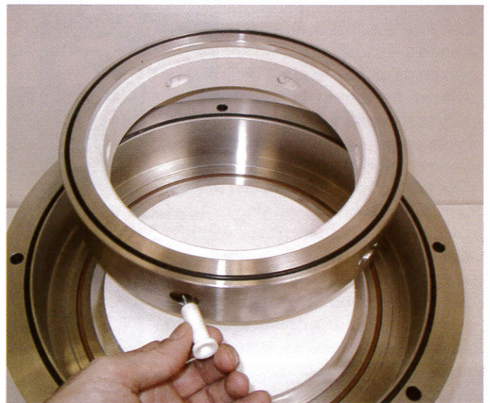
Figure 7. In the open-manifold jet mill, jets are easily removed without access ports.
