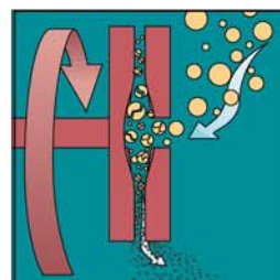
Sample Grinders: Disk type grinder for very fine work at small throughput rates.
