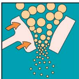
Jaw Crusher: Ideal for coarse and intermediate crushing; minimal fines production.
