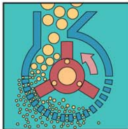
Hammermill: Versatile, perfect for friable materials; easy access for maintenance or inspection.
